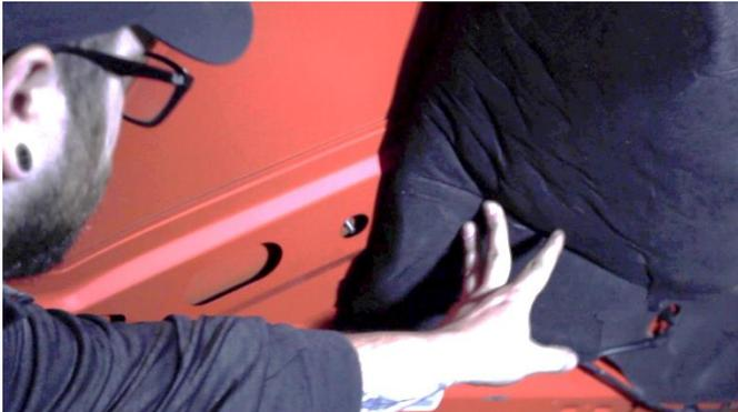
With a 10mm socket, hold the bumper with one hand and unscrew and remove the nut. Repeat on the opposite side.
