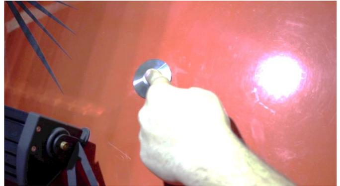
With the other, secure a washer and a nut to the countersunk bolt. With a 13mm socket and 5mm allen key, tighten the nut and repeat on the opposite side.
