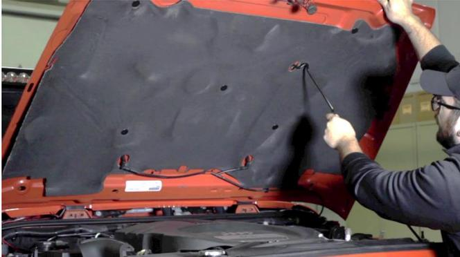
Peel back the heat shield enough to gain access the hood bumper nuts.
