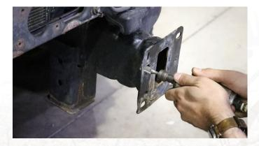
In the back of the bumper, install 2 of the nut plates into the outboard bumper-to-frame brackets, and screw on the included plastic washers to help keep them in place.
