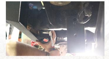
With the 2 flanged bolts and hex nuts, secure the bottom of the winch plate.
