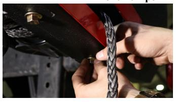
Install the two trim accents with the small nutplates and small nyloc nuts with a 5mm socket.
