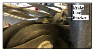
6. Remove brake line bracket bolt with 12mm wrench to take tension off brake line then lowering axle
