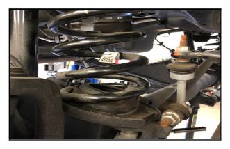
8. Compress spring down if necessary install new coil spacer, OE spring isolator and reinstall spring. Be sure to line up the previously applied coil spring reference mark, install bolt and supplied lock nut.
