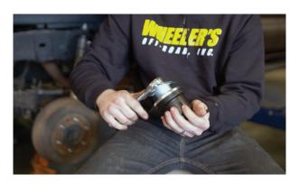
**7.** Install bumpstop on flip plate as shown with supplied hardware.
