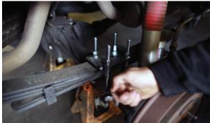
**4.** Cut excess U-bolt material approximately ½" above the nut.
