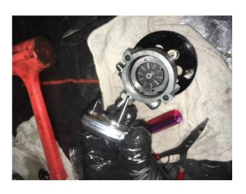
This photo shows improper retaining ring install, if installed correctly your pump WILL NOT look like this
