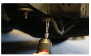
**19.** Remove rearmost hanger from exhaust pipe.
