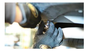
**4.** Remove bolts and clips from lower inner fender/ mudflap.
