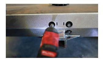
**24.** Loosely install side support on bumper as shown. Supplied bolt will install in factory location shown.qa
