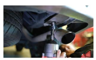
**23.** Adjust fit of bumper and tighten hitch mount bolts and lower frame rail bolts.
