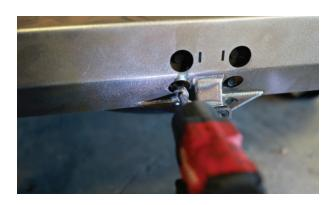
**22.** Loosely install supplied bolts and washers into the two bolts on the bottom of each frame rail.
