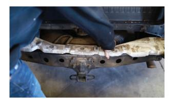
**16.** Using a rubber mallet knock spare tire stops down until they are approximately one inch above the bumper cross member. Spare tires needs to be lowered for this step.
