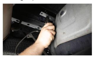
**10.** Attach the secondary mounting bracket to the top of the passenger mounting bracket using the supplied hardware as shown. Tighten this bolt.
