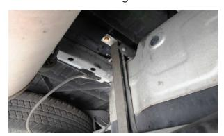
**11.** Tighten all installed bolts. DO NOT exceed 33 ft-lbs when tightening the front bolts going into the nut plates.
