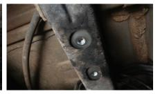
**3.** While supporting the new skid plate, align the front mounting holes with the clinch nuts and start (2) of the supplied mounting bolts with washers. Do not fully tighten these bolts yet.
