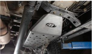
**1.** If equipped, remove the factory fuel tank skid plate by loosening and removing the (4) mounting nuts.
