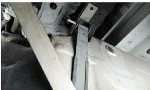
**9.** If needed, bend the tabs on the tank mounting strap outward.
