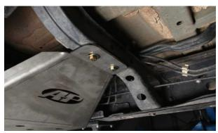
**4.** Install the rear driver and passenger skid mounts onto the skid plate as shown using the supplied hardware. The passenger mount is the longer mount and the driver mount is the short mount. Do not fully tighten these bolts yet.
